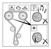
The control valve filters are clogged due to dirt and abrasion. As a result, the camshaft phasing units are not supplied with sufficient engine oil and are irreparably damaged. This damage is evident in the form of a significant noise generation and/or oil leakage.
