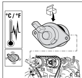
The central magnet is subject to vibration and thermal loads. In order to prevent a fault, this magnet should also be replaced during the repair.
