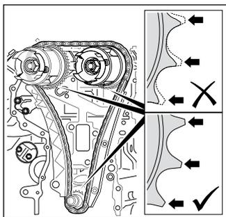
Over time the toothed gears (on the crankshaft/camshafts) may become worn, which can lead to engine damage. For this reason, it is recommended to replace the complete timing drive.
