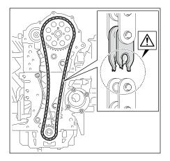
Wear can cause the timing chain to lengthen, which can lead to the chain jumping or, in the worst case scenario, breaking. In addition to damaging the complete timing drive, this usually also causes damage to the valve train.
