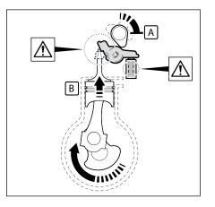
If, once the chain has broken, the camshaft is no longer driven by the crankshaft [A], the valves remain partially open. The valves are pressed against the finger followers by the pistons [B]. The pistons may also strike the valves if the chain jumps.
