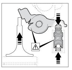
As the finger followers are not able to move out of the way, they become deformed. Due to the high load, the hydraulic pivot elements also become damaged (not visible from the outside). The camshaft is not usually damaged. In-depth testing for any additional resulting damage is obligatory, in particular damage to the valves.
