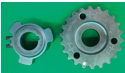
Fuel Injection Pump Sprocket
