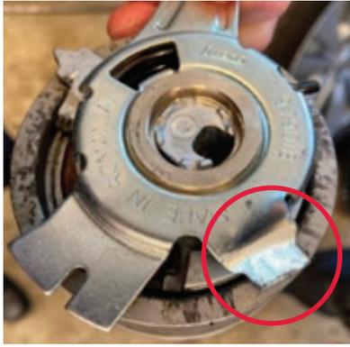
**Tensioner failure tab damage**
