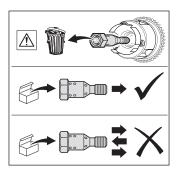
The threaded part of the central valve stretches during assembly and therefore must not be re-used after removal.
