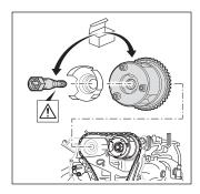
The central valves and camshaft phasing units supplied in the INA Engine KIT must always be used.
