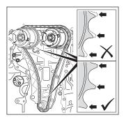
Over time the toothed gears (on the crankshaft/camshafts) may become worn, which can lead to engine damage. For this reason, it is recommended to replace the complete timing drive.
