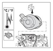
The central magnet is subject to vibration and thermal loads. In order to prevent a fault, this magnet should also be replaced during the repair.
