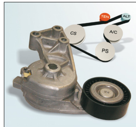
Image 2: Tensioner lever 534 0132 30 installed in 1.9 TDI engines with belt path
