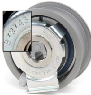
Photo 1: 531 0777 10 – Old tensioner pulley (979743)
