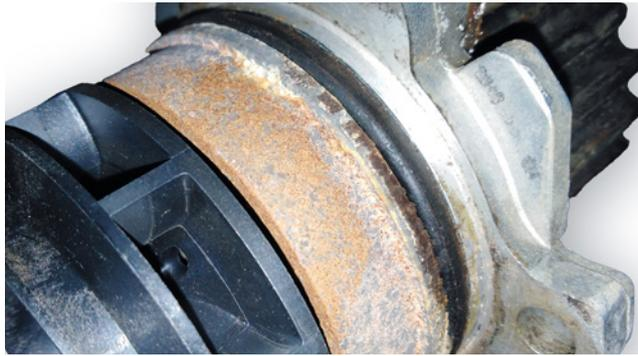
Figure 1: Signs of corrosion on a coolant pump
