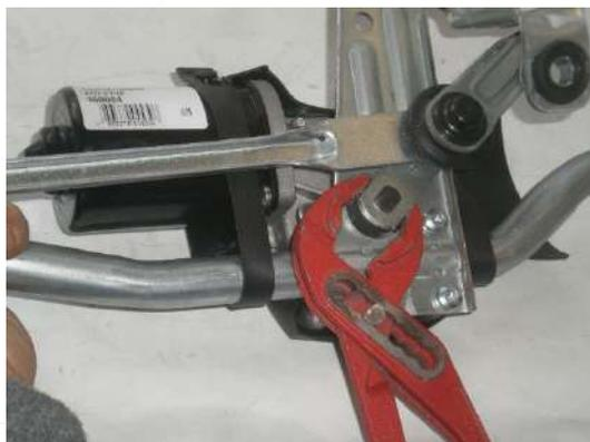
3) Rotate the output lever until the four screws are visible.
