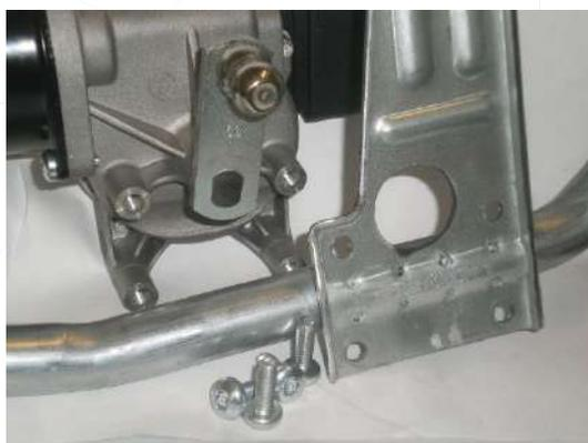
In circled image is visible one of the new wiper motor OE fitting holes, without thread. The motor mounting holes have no thread because the fixing bolts are self-tapping.
