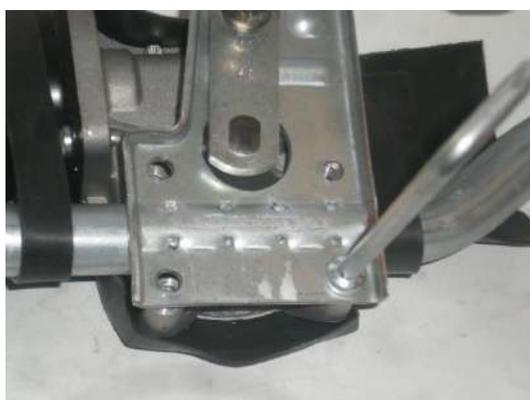
6) Remove the motor from the bracket
