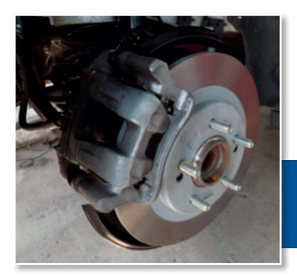
In order to remove the caliper carrier (A), first remove a suspension link bolt (B). This will enable you to remove the two caliper carrier bolts (C).
