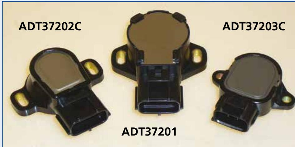
This device signals the exact position of the throttle valve at any time to the engine ECU by varying the output voltage through a variable resistor or potentiometer. It is a key component in the vehicle engine management system and if malfunctioning may cause symptoms such as;
