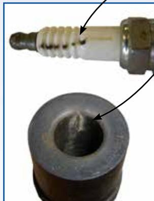
**Example B** shows where the spark has tracked along the spark plug ceramic (see burn marks).
