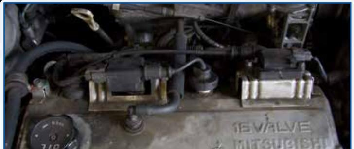
Blue Print strongly recommend that the spark plugs and HT leads are replaced in addition to the coil assembly, or that they are carefully checked. We also recommend that a logical diagnosis procedure is followed (prior to replacing the ignition coil) to prevent it being replaced unnecessarily.
