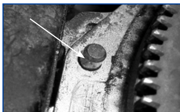
Gearbox location dowels (missing or damaged)
