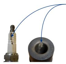
**Example B** shows where the spark has tracked along the spark plug ceramic (see burn marks).
