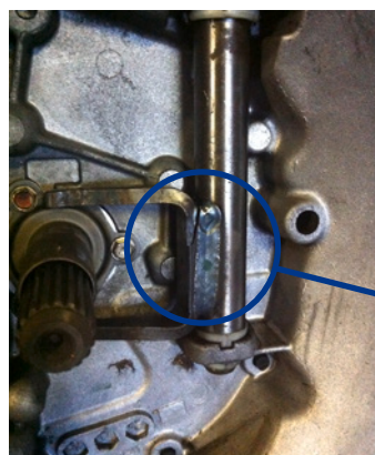
CLUTCH FORK FRACTURE
