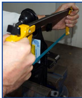
2. Using a hacksaw, cut through the bracket vertically as close to the welded flange as possible.
