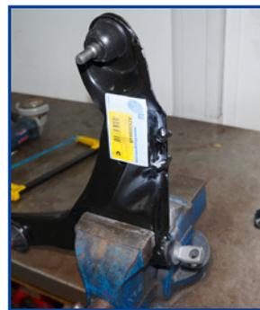
3. Using a file or hand grinder, remove any burrs or sharp edges.
