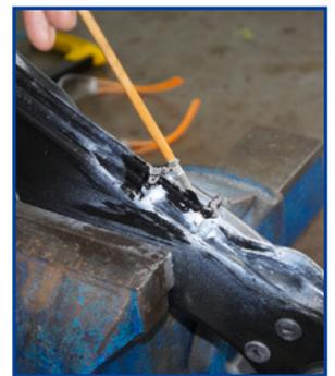
4. To protect against corrosion it is necessary to cover the exposed bare metal. Apply a layer of primer to the bare metal. Then once dry, apply a coating of an oil based paint. Alternatively use a good quality stone-chip guard type paint.
