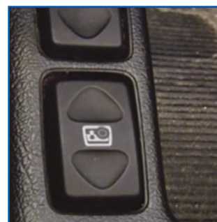
The tailgate window switch is located in the centre console near the handbrake.
