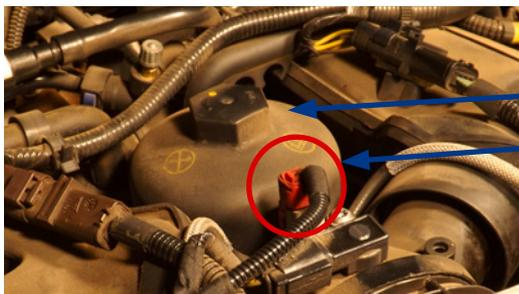
On removal of the engine cover, you will find the oil filter element housing in the centre of the engine at the top.
