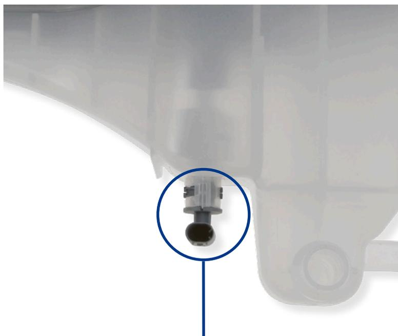
On replacement of the expansion tank, top up with the correct coolant and check for leaks from the coolant hoses after refitting and ensure you connect the level sensor.
