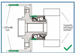
1. This kind of hub assembly needs to be installed with special tools to avoid damages to the inner structure of the bearing. The force has to be applied on the outer ring of the bearing urgently. Otherwise with initial effect the product will make noise, can get play and the lifetime will be shortened immediately.
