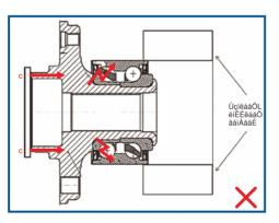
As shown on the picture, wrong force application will damage the inner structure and lead to the problems mentioned above.
