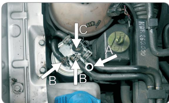
(EN) Install filter in clamping ring; fasten the screw (A). Fix hoses (B), regulation valve and fastening clamp (C)
