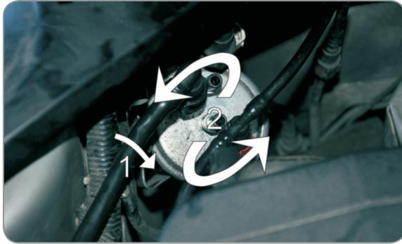
(EN) Take fuel filter off the bracket. Remove fuel filter fastening clamp. Turn the fuel filter anti clockwise. Take fuel filter off the bracket
