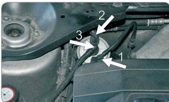
(EN) Disconnect fuel pipes from fuel filter in a sequence shown in the picture
