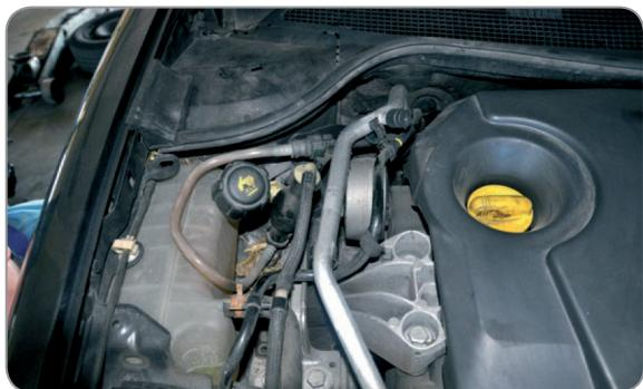
Pump with manual pump till resistance is felt, start the engine, check for leakage
