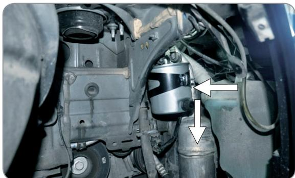
Install fuel heater valve element, fuel hoses and place filter in seat
