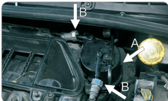
**EN** Disconnect the fuel heater connector placed in bottom part of filter (A) open the quick connects of fuel hoses (B), remove filter\*
