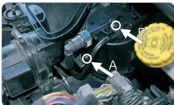
**EN** Fasten screw fastening fuel filter (A) and screw fastening the brake vacuum pipeline (B)
