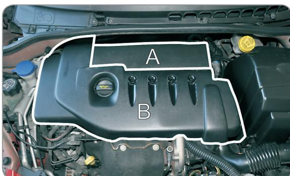
**(EN)** Remove air filter cover (A), remove engine masking frame (B)
