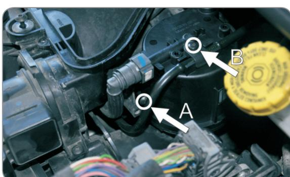
**(EN)** Unscrew the screw fastening fuel filter (A) and screw fastening the brake vacuum pipeline (B)
