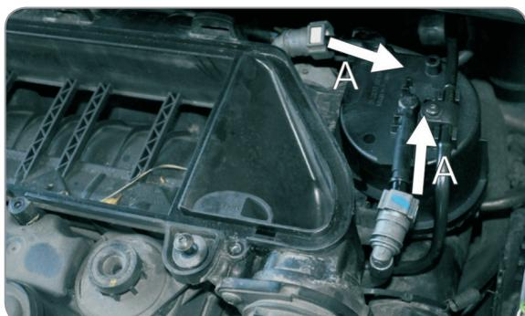
**EN** Connect fuel heater connector, fix new filter in casing and then remove plugs and connect fuel hoses (A)\*\*
