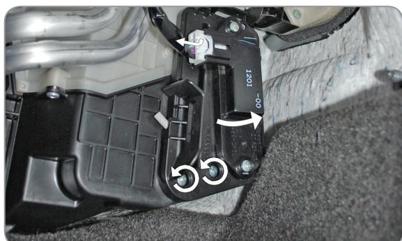
**EN** Disconnect the electric circuit, loosen the screws that hold the cover itself
