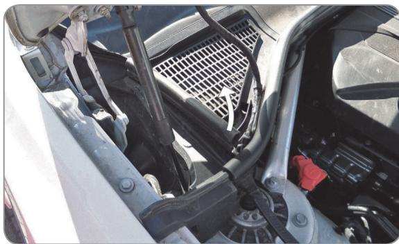
(EN) Remove the rubber seal
