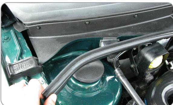
**(EN)** Remove the rubber seal
