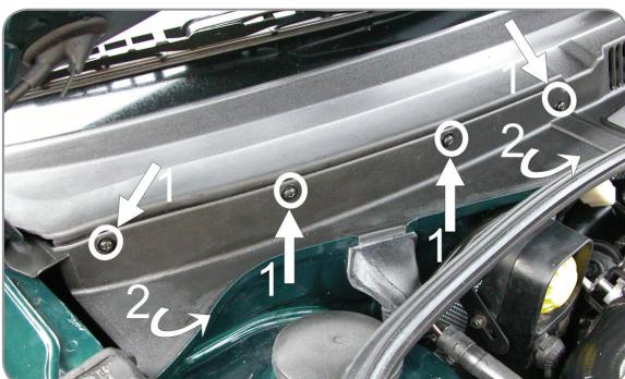
**(EN)** Loosen the screws on the filter housing. Remove the filter housing
