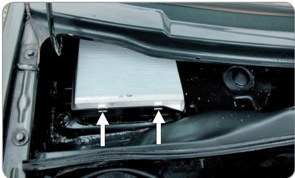
**(EN)** Unlatch the filter from its socket
