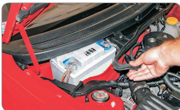
(EN) Remove the rubber seal
