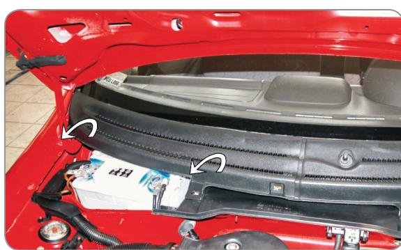
(EN) Remove the first section of the screen
