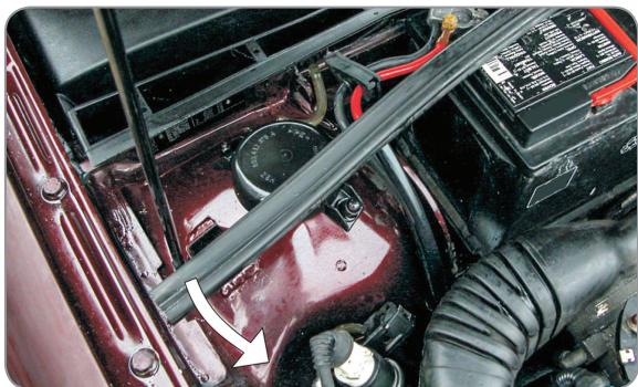
**EN** Remove the rubber seal
