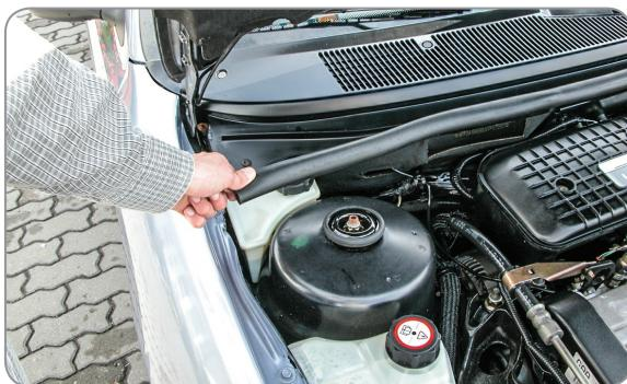
EN Remove the rubber seal
