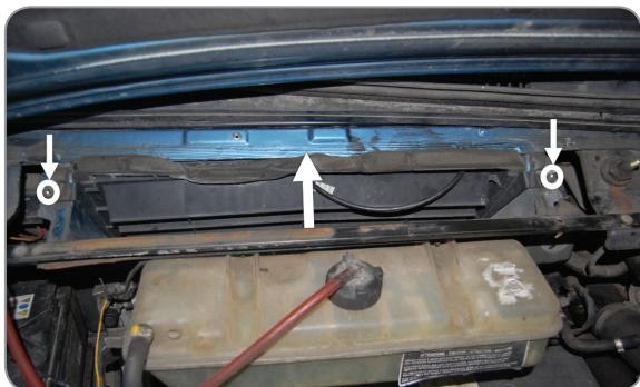
EN Take the filter out together with the frame
