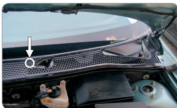
(EN) Take out the screen section and turn off the screw from it
