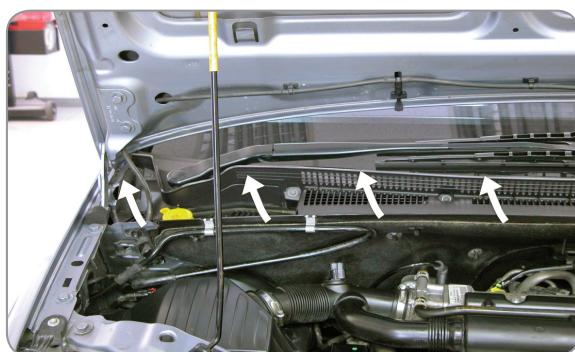
(EN) Remove the rubber seal
