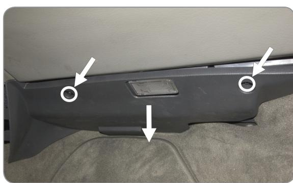
(EN) Loosen the screws and remove the upper wall of the locker.
