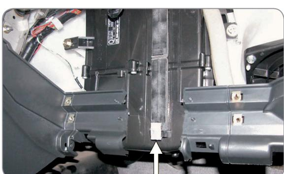
**EN** Remove the filter fastener
