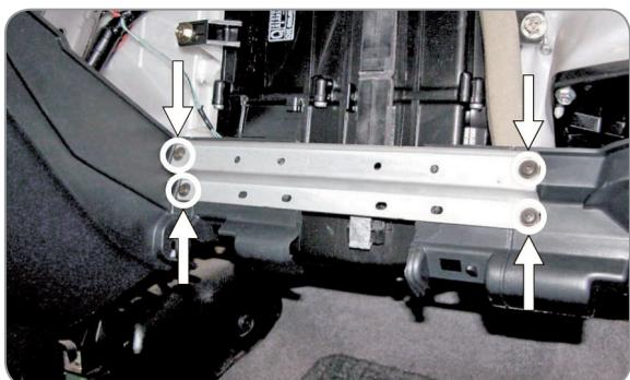
**EN** Remove the protecting device
