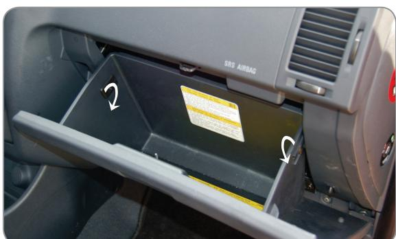
**EN** Remove the glove compartment
