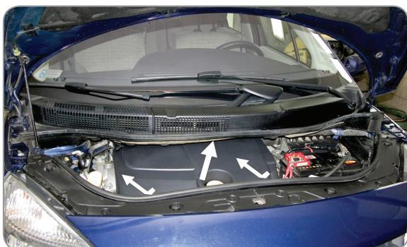
EN Remove the engine housing
