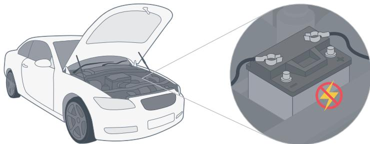
To minimise the risk of damaging electronic subcomponents in the steering rack, both battery terminals on the vehicle must be disconnected.
