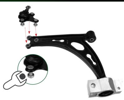
ENSURE BOLTS ARE TIGHTENED TO MANUFACTURER SPECIFICATION
