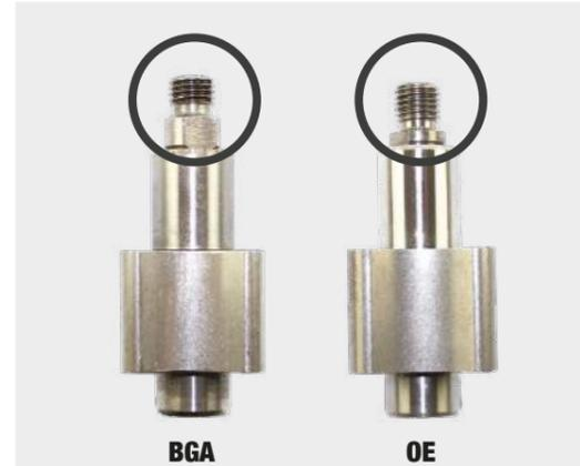
A design flaw in the OE Pump led to insufficient contact area between the drive shaft and the rotor, allowing  $3-5^\circ$  of movement between the shaft and the rotor. BGA reengineered the shaft to increase this surface area by 72%.
