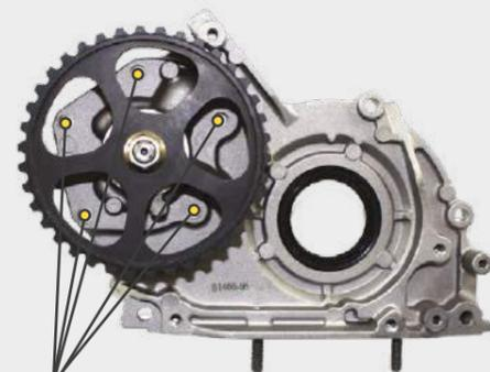
The bolt holes are accessible; Pulley removal is not necessary.
