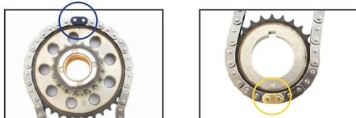
2.2. Align camshaft dowels and timing marks.
