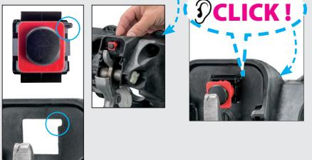
(UK) 5. Connect the electrical connector and slowly release the brake pedal to allow the switch to self-adjust.
