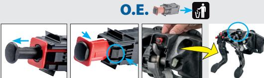
(UK) 1. Disconnect the electrical connector, extract the (red) lock bushing completely, press the retaining clips and remove the switch to be replaced.
