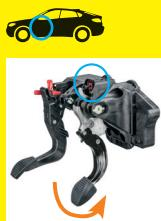
(UK) Perform all switch disassembly and assembly operations with the brake pedal pressed down.
