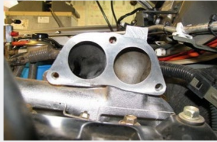
Clean intake manifold
