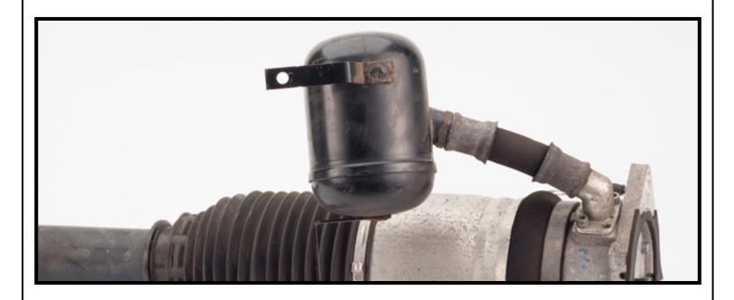
THE ARNOTT REMANUFACTURED STRUT DOES NOT REQUIRE THE REUSE OF THE EXISTING RESERVOIR. DO NOT ATTEMPT TO REMOVE AND FIT TO THE ARNOTT PRODUCT.
