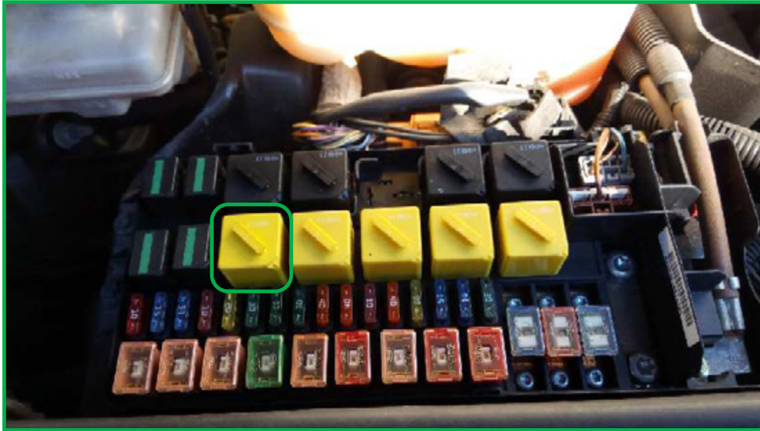
98-04 LAND ROVER DISCOVERY II (L318) Relay located within Underhood Fuse Block.
