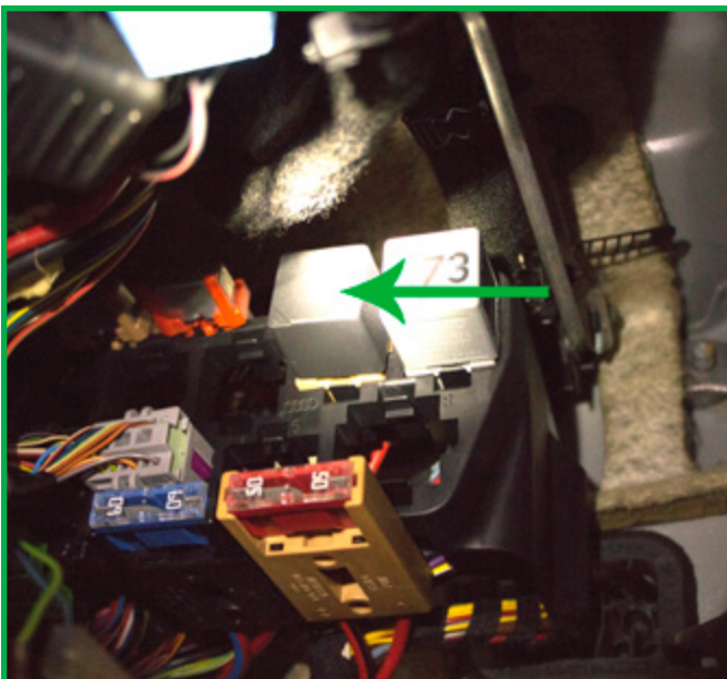
01-05 AUDI ALLROAD QUATTRO (C5) Relay located on the left side of the vehicle under the dashboard.
