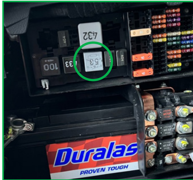
03-19 BENTLEY CONTINENTAL GT/06-19 FLYING SPUR (D1) Relay located in rear left of the trunk, above the battery.
