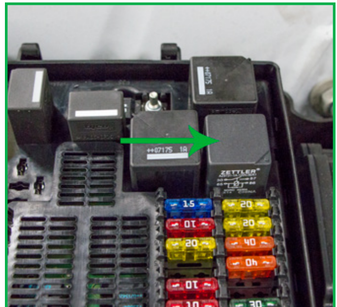
04-09 JAGUAR XJ SERIES (X350/358) Relay located on the right side of the vehicle in the engine compartment.
