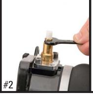
TIGHTEN FITTING TO APPROX. 2NM (18 IN-LBS/1.5 FT-LBS)
