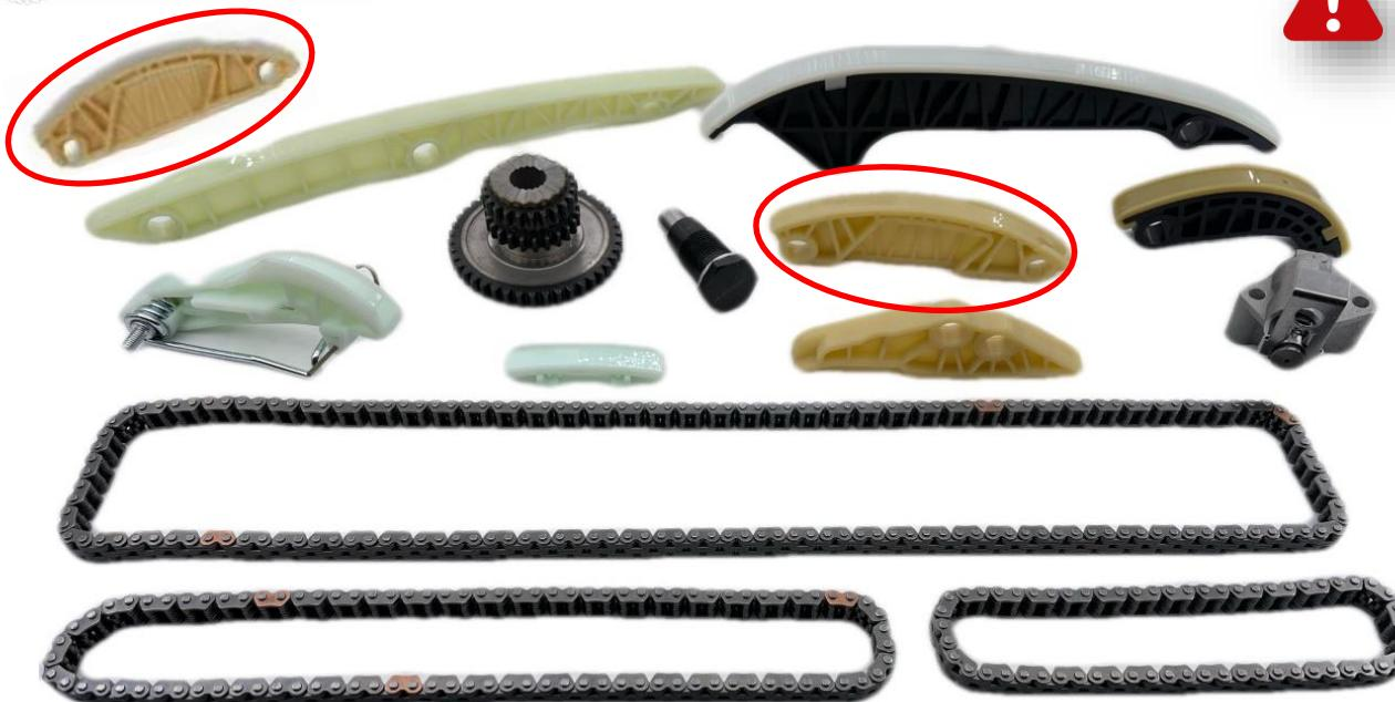
Check that the guide that you removed matches one of this kit. The guide (06H109469AN) for the new EA888 VAG engine is a little longer than other engines guide (06H109469AQ).
