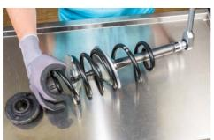
• After extraction, relieve the tension on the spring and remove the tools.
