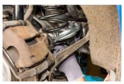
Insert the upper tensioning jaw into the upper part of the spring and thread the spindle. The pendulum 6-point head must now be in the hexagonal guide of the tensioning jaw.
