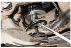
If, after being inserted into the axle, the spindle nut cannot be reached with the tubular box wrench, the spindle nut of the safety spring vice must be relieved of tension with a combination wrench SW 24 through the spring windings.
