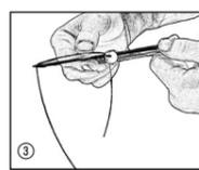
③ Insert the wire from the top through the opening at the knurled screw.
