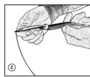
④ Press the end of the wire to the tool shaft.
