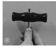
④ Press the end of the wire to the tool shaft and pull the shaft through the handle.
